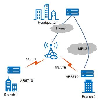
Huawei NetEngine AR6710-L series routers feature 5G/LTE functionality, enabling wireless interconnection between enterprise branches and between the headquarters and branches. A 5G/LTE link can function as the active link or as a backup for wired links, enhancing network stability while reducing network construction cost.
