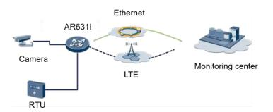
Huawei AR631I-LTE4EA can be deployed to provide 4G/3G wireless backhaul for cameras in areas where conventional wired coverage is difficult. It can also offer 4G backhaul in industrial manufacturing scenarios. Due to highly reliable industrial design, AR631I-LTE4EA ensures secure and reliable network communication in challenging environments with extreme temperature, humidity, and electromagnetic interference.
